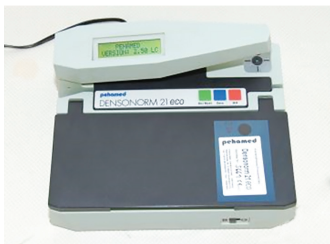
Fig. 3: Transmission densitometer used in the present study
