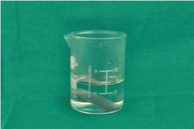
Fig. 1: Acid etching of titanium plate
