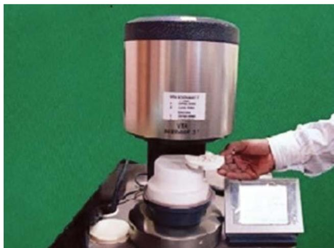
Fig. 3: Blocks kept in Zirconia furnace for sintering
