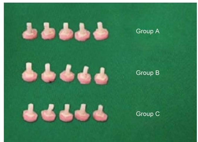
Fig. 7: Composite cylinders cemented on all the 15 Zirconia samples
